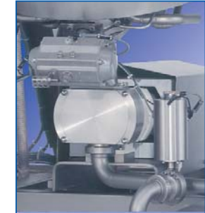
Recirculating / discharge pump
